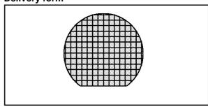
The ST16CF54 can be delivered either in unsawn or sawn wafers, 180 or 275 micron thickness.
